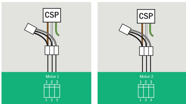
**ENGLISH:** To ensure cable monitoring, relocate the terminal module (prefitted in the terminal block in the control system); connect terminal module and CSP cable to power cable. The cables must not be transposed; this would cause malfunction of the terminal module.
