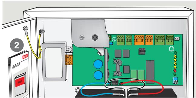
**ENGLISH:** Position the label supplied, SMOKE VENT, on the front of the control system as shown ①. Keep instructions on the inside of the door ②.
